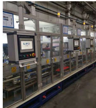
04 Grinding & honing Automatic grinding lines finish raceways and rollers.
