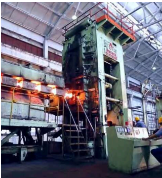
01 Forging Automatic forging lines shape the rings from bearing-steel bar.
