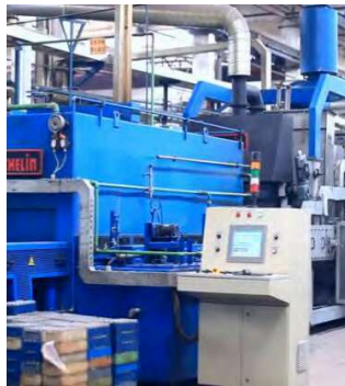
03 Heat treatment Continuous gas carburising and controlled-atmosphere die quenching.
