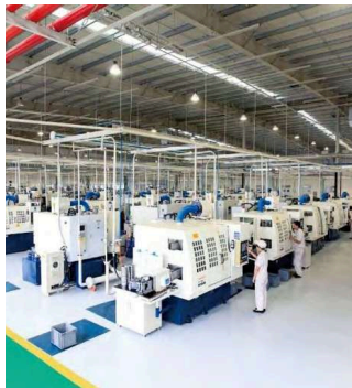
02 Turning CNC turning to near-net shape, ring by ring.
